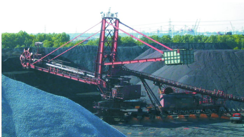
Fig. 1: Combined stacker reclaimer handling raw materials
